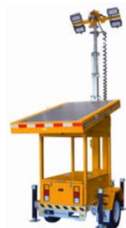
Solar Light Tower
